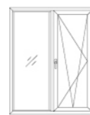
Inward opening and tilting inward
