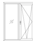
Inward opening and tilting inward
