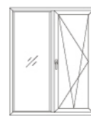
Inward opening and tilting inward
